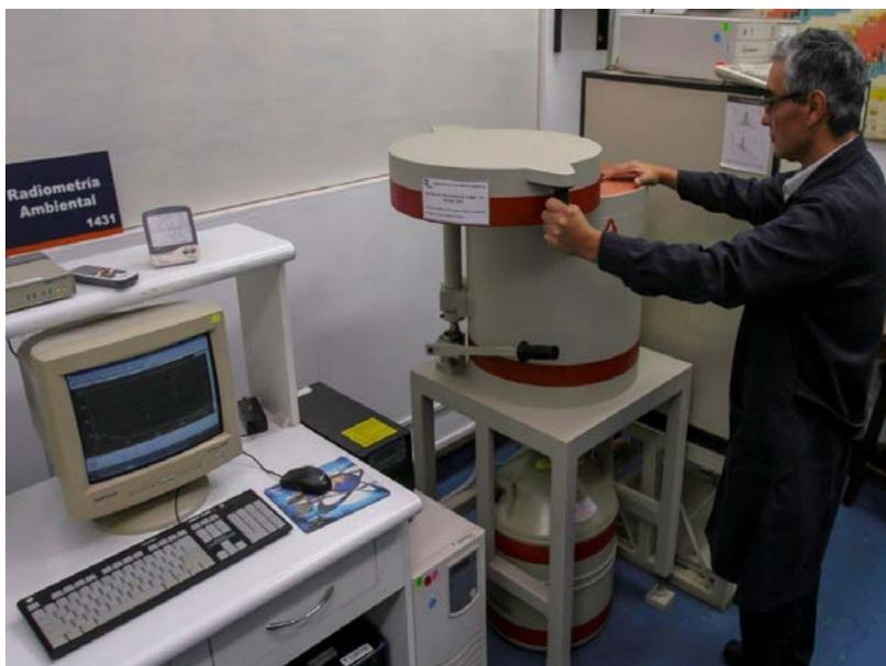
Figure 3. Gamma spectrometry system.
