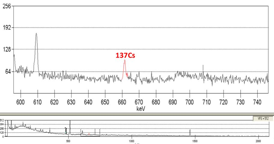
Figure 4. Gamma spectrum of <sup>137</sup>Cs.
